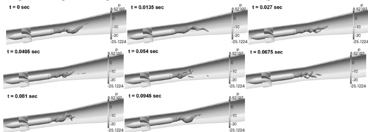
Fig.9 Numerical calculated time evolution of the vortex structure
