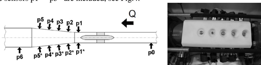
Fig.4 The pressure sensors arrangement (left) of experimental measurements (right)
