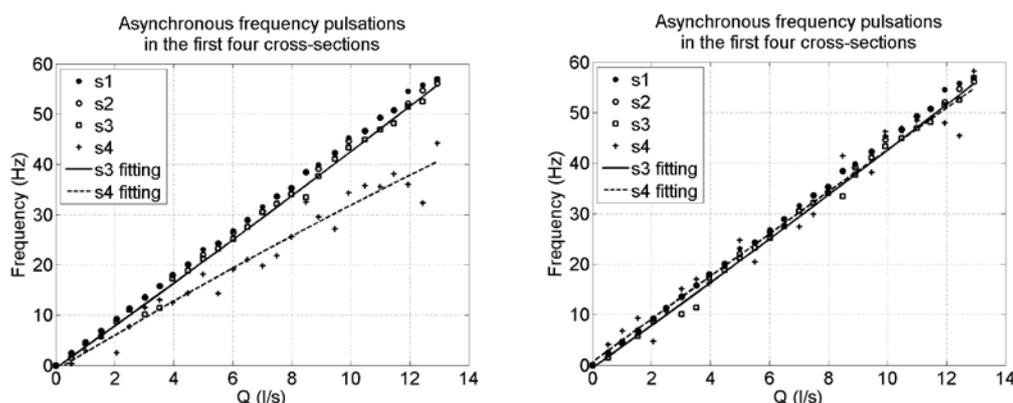
Fig.7 The frequency values of asynchronous pressure pulsations in the third and the fourth cross-sections treated by diameter growth ratio (left) and in the fourth cross-sections treated by influence of synchronous pulsations (right)
