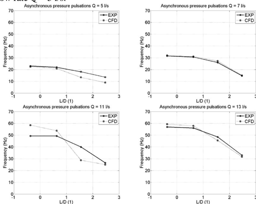
Fig.11 Frequency of asynchronous pressure pulsations (EXP) vs. calculation (CFD)
