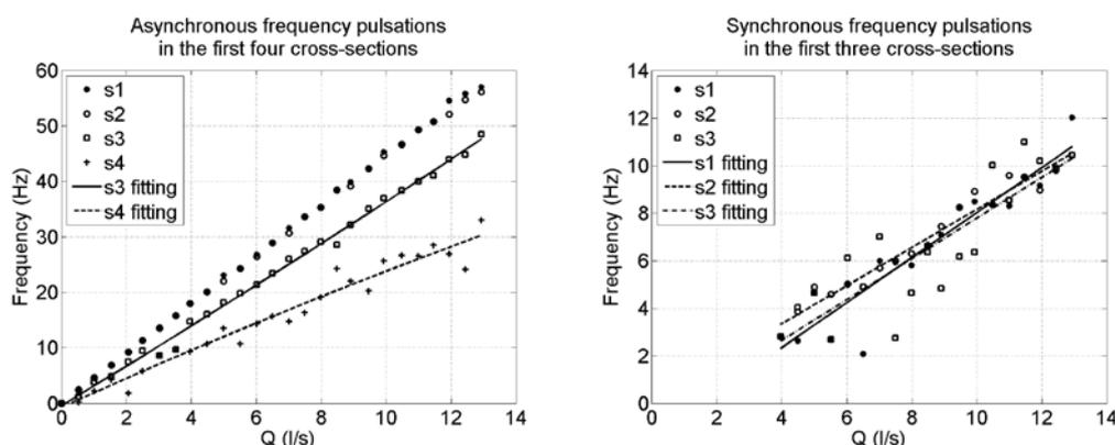
Fig.6 Asynchronous (left) and synchronous (right) pressure pulsations
