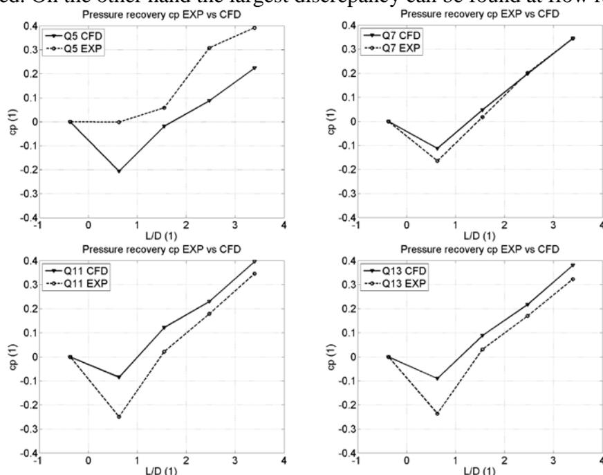
Fig.10 Pressure recovery factor experiment (EXP) vs. calculation (CFD)
