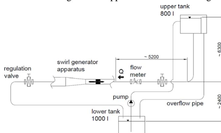
Fig.3 Scheme of experimental test rig
