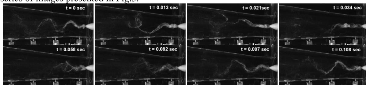
Fig.5 The experimental observation of the spiral vortex time evolution
