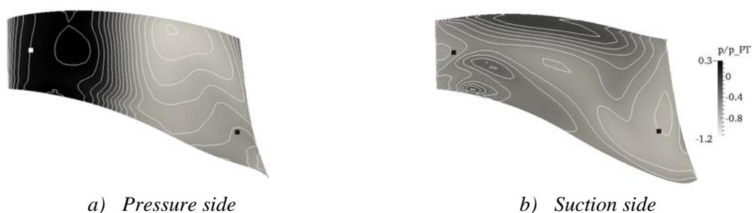
Fig.5 Pressure distribution at  $t = 5$  s in pump break mode. Pressure difference between contour lines corresponds to 10 % of envisaged head over the machine. Pressure evaluation points are marked with dots.
