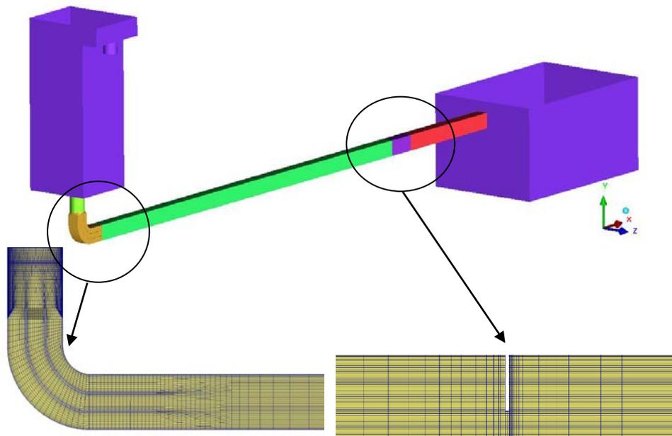
Figure 5: Computational domain and some features of the mesh.
