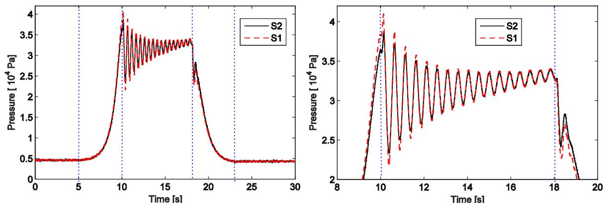
Figure 2: Pressure variation recorded at the two sensor positions upstream the gate.
