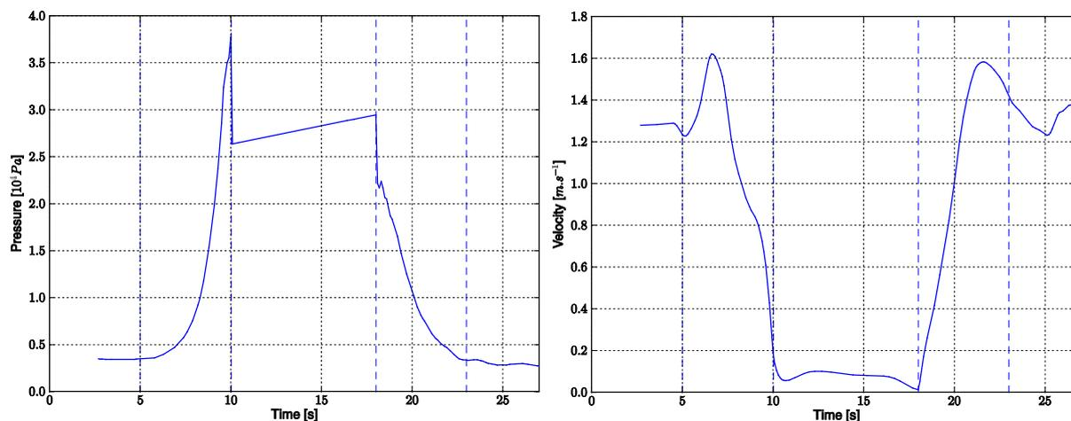
Figure 7: 3D computed pressure (left) and velocity (right) upstream the gate.
