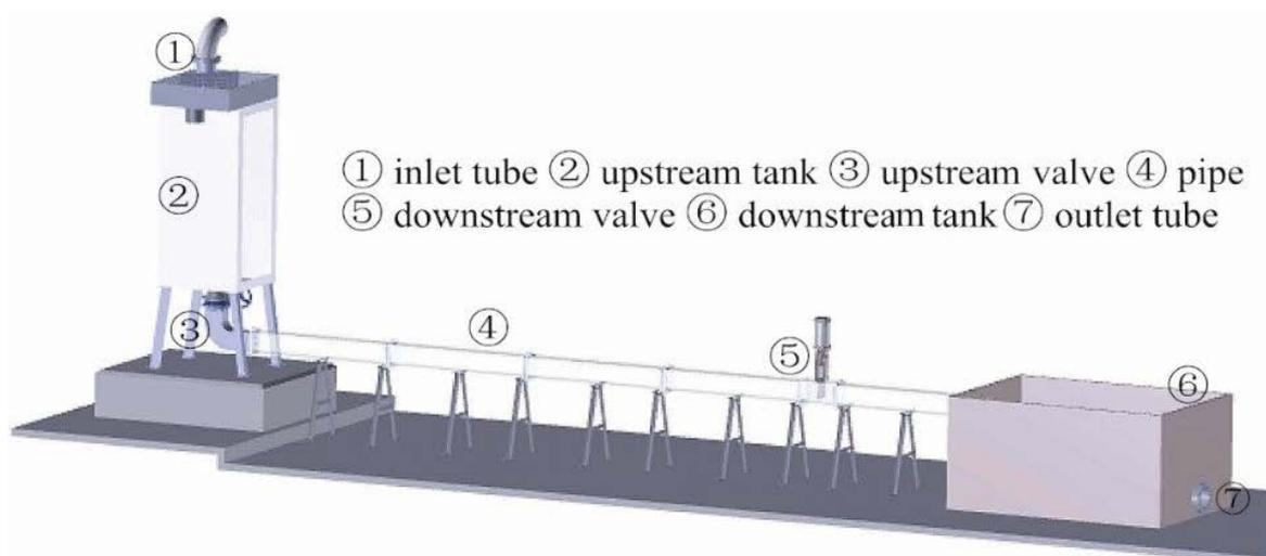
Figure 1: Layout of test rig
