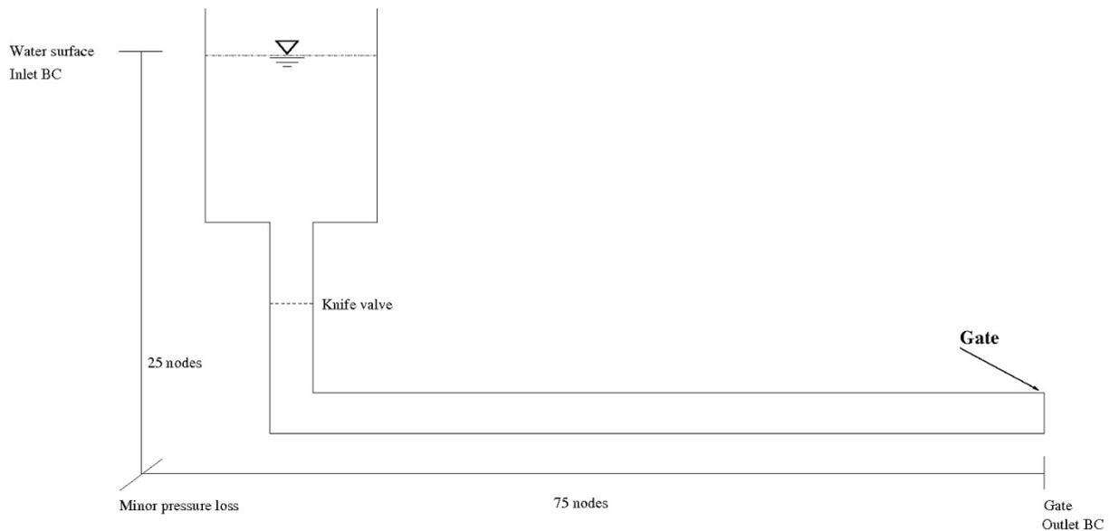
Figure 9: Computational domain for the 1D MOC computations.
