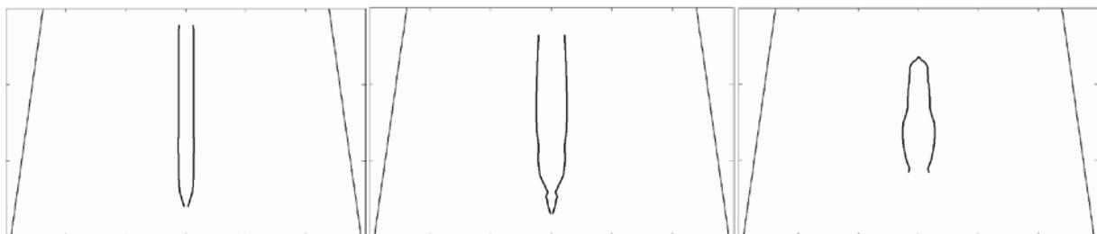
Fig.5. Forms of calculated cavitation bubbles in the draft tube
