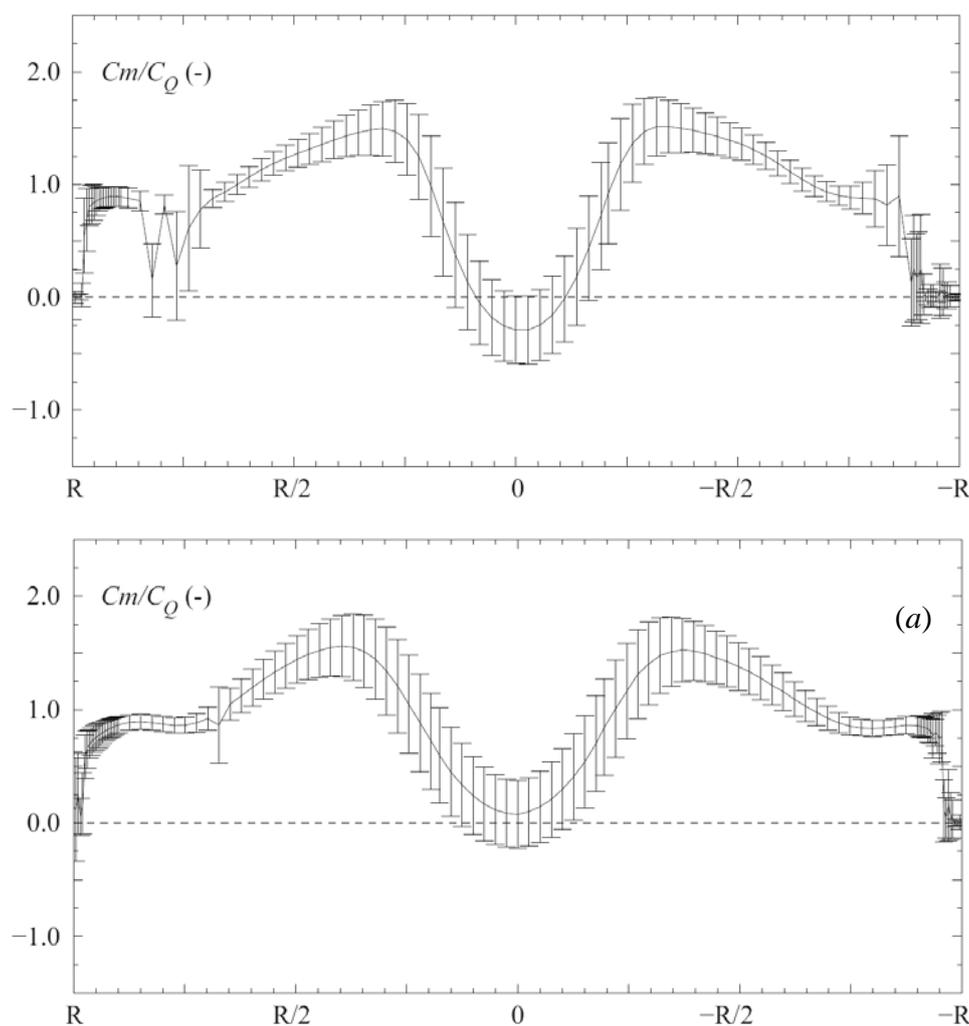
Fig.2. Profiles of the axial velocity component  $C_m$  at the BEP [2] at Section 1 (a) and Section 2 (b)
