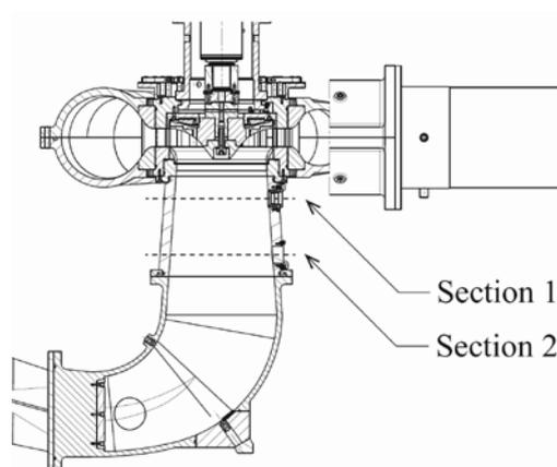
*Fig.1. View of the reduced scale model. Section 1 and Section 2 for LDV measurements are located  $0.39 \times D_1$  and  $1.0 \times D_1$  below the runner exit*
