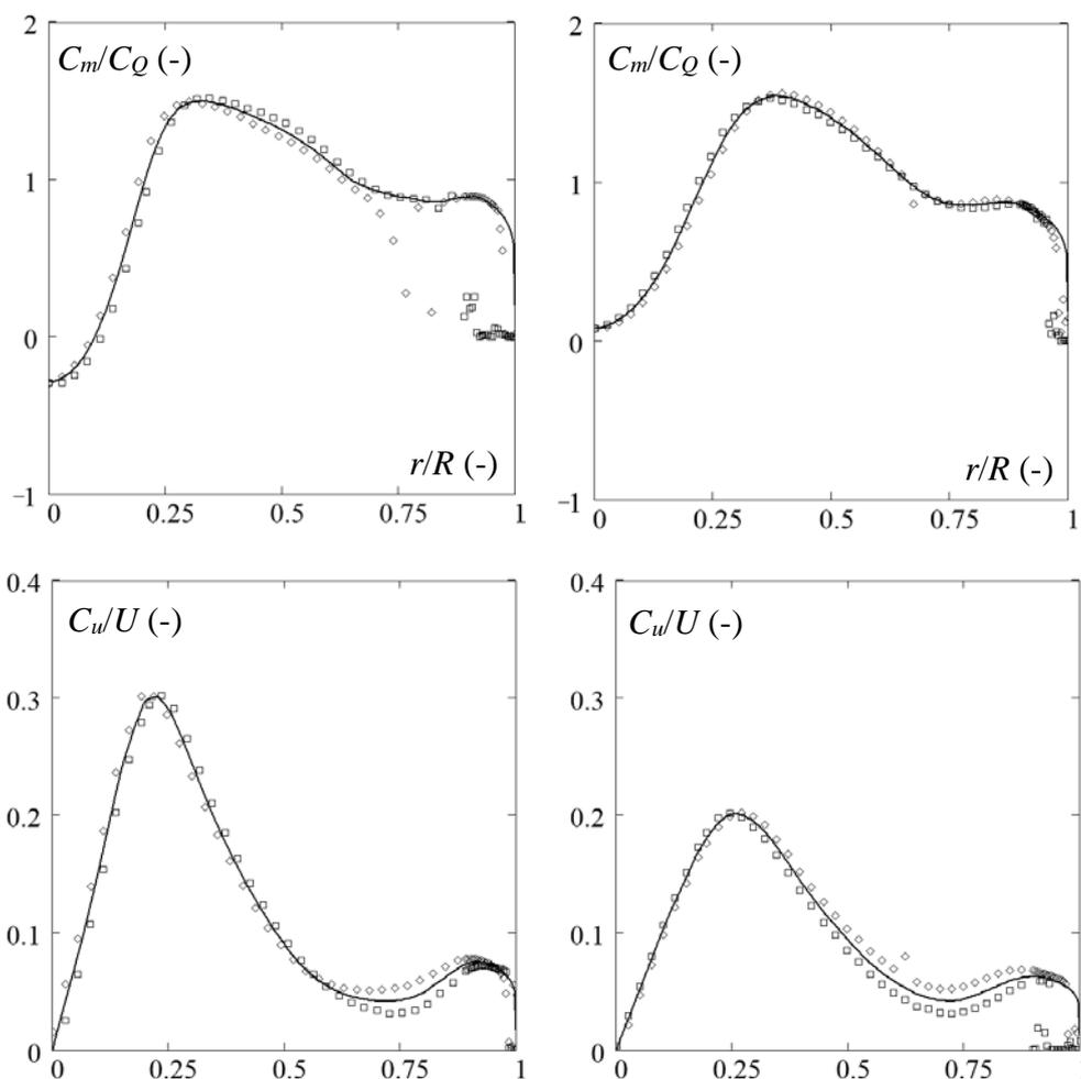
Fig.4. Symmetrized and smoothed profiles of the axial (a, b) and tangential (b, c) velocities in Section 1 (a, c) and Section 2 (b, d) of the draft tube. Symbols correspond to the measurements data from [2].
