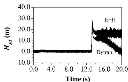
Fig. 3 Comparison of heads at the position 3/3 measured by Dytran and E+H pressure transducers: pipeline filling
