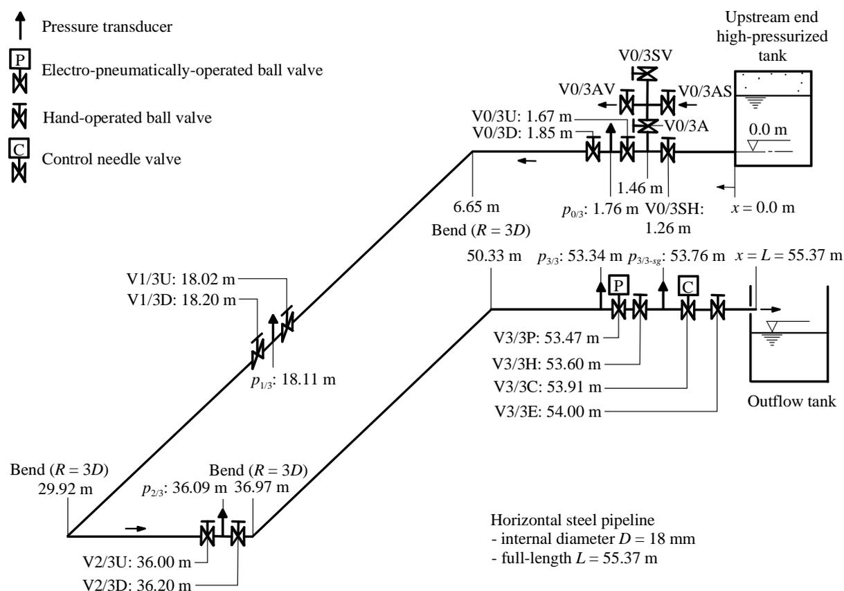
Fig. 1 Layout of small-scale pipeline apparatus
