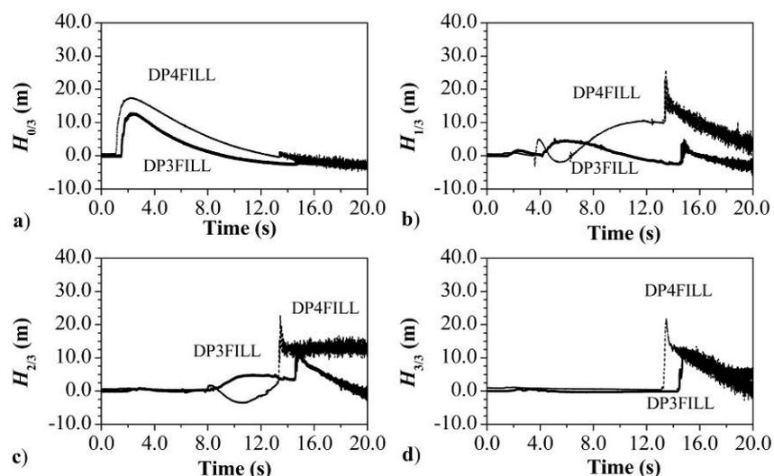
Fig. 4 Comparison of heads at the end valves ( $H_{3/3}$  and  $H_{0/3}$ ) and along the pipeline ( $H_{2/3}$  and  $H_{1/3}$ ) for the different pressure values: pipeline filling
