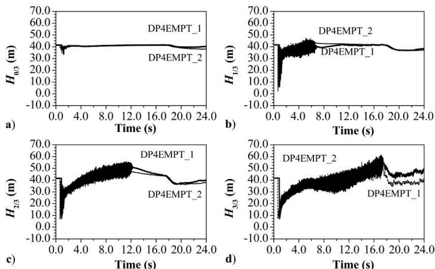
Fig. 5 Comparison of heads at the end valves ( $H_{3/3}$  and  $H_{0/3}$ ) and along the pipeline ( $H_{2/3}$  and  $H_{1/3}$ ) for the same initial conditions: pipeline emptying
