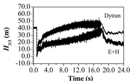
Fig. 6 Comparison of heads at the position 3/3 measured by Dytran and E+H pressure transducers: pipeline emptying
