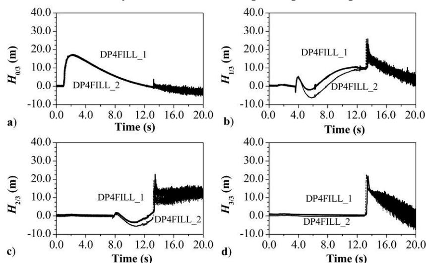
Fig. 2 Comparison of heads at the end valves ( $H_{3/3}$  and  $H_{0/3}$ ) and along the pipeline ( $H_{2/3}$  and  $H_{1/3}$ ) for the same initial conditions: pipeline filling
