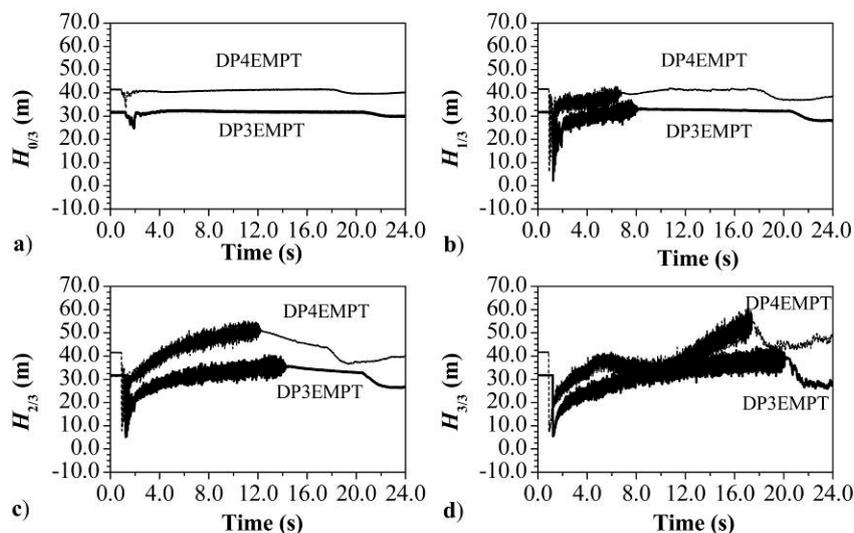
Fig. 7 Comparison of heads at the end valves ( $H_{3/3}$  and  $H_{0/3}$ ) and along the pipeline ( $H_{2/3}$  and  $H_{1/3}$ ) for the different pressure values: pipeline emptying
