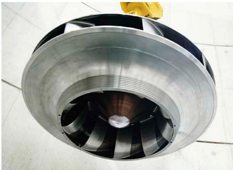
Fig. 1: Picture of a pump turbine runner
