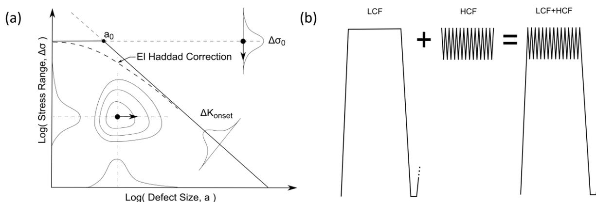
Fig. 1 (a) Fatigue reliability limit state; (b) Structure response spectrum.
