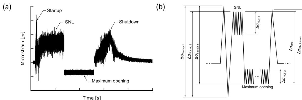
Fig. 7 (a) Measured example of Type 2 response; (b) Type 2 simplified response spectrum.
