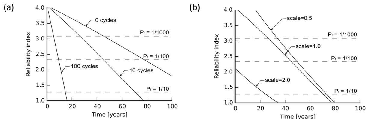
Fig. 8 Case 3 sensitivity analysis; (a) Number of cycle  $N_{HCF1}$ ; (b)  $\Delta\sigma_{HCF2}$  uncertainty (i.e.: scale).
