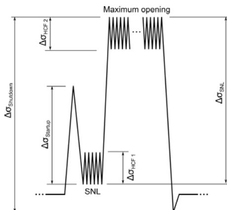
Fig. 2. Type 1 simplified response spectrum.
