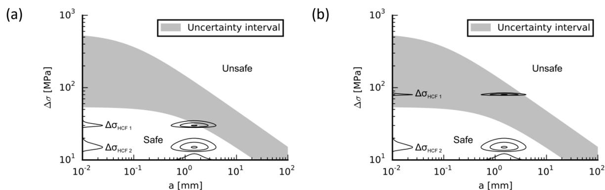
Fig. 6 (a) Case 2 with all operating condition safe; (b) Case 3 with some operating condition unsafe.
