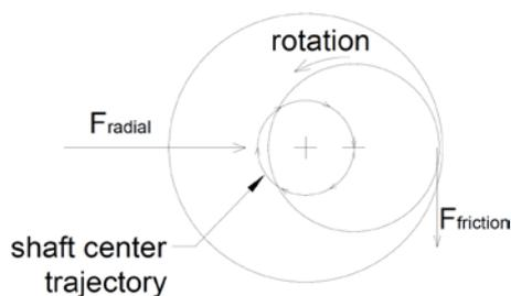
Fig. 9: Schematic diagram of forces in the bearing
