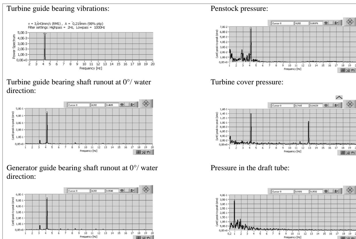
Fig. 5: Frequency specter in measured signals
