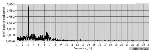
Fig. 4: Frequency analysis of the shaft runout signal in unit mechanical run
