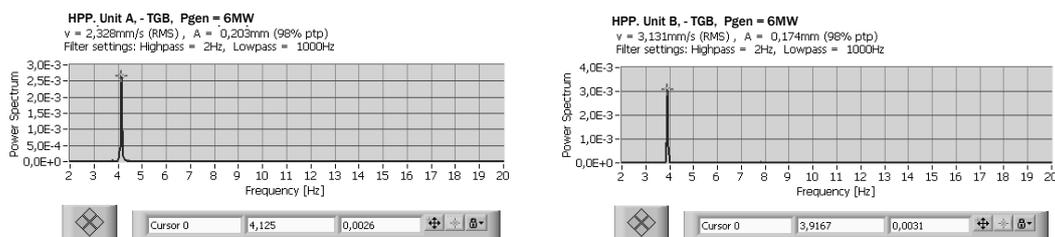
Fig. 2: Radial vibrations measured at the turbine guide bearing (unit A and unit B)
