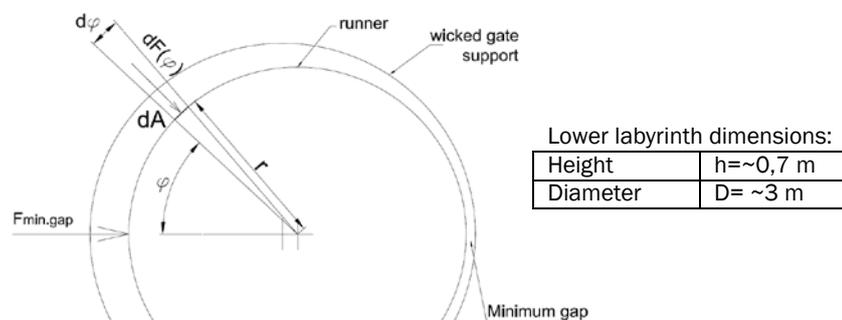
Fig. 14: Schematic of forces in the lower runner labyrinth
