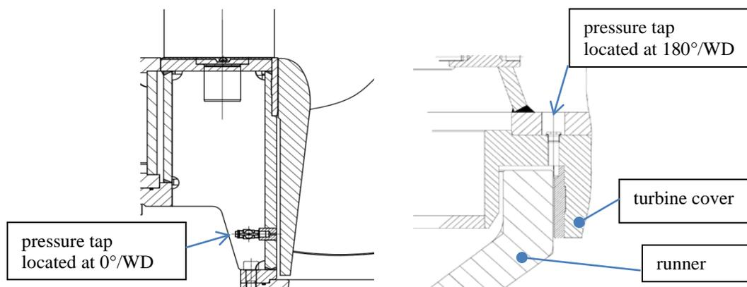
Fig. 10: Location of pressure measurements in the runner labyrinths
