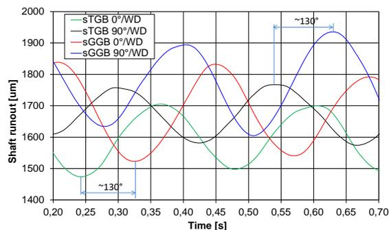
Fig. 7: Shaft runout raw signal data measured at 17MW (75% load)
