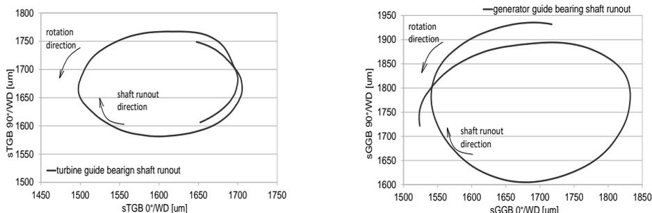
Fig. 8: Shaft runout orbit measured on the turbine and generator guide bearing
