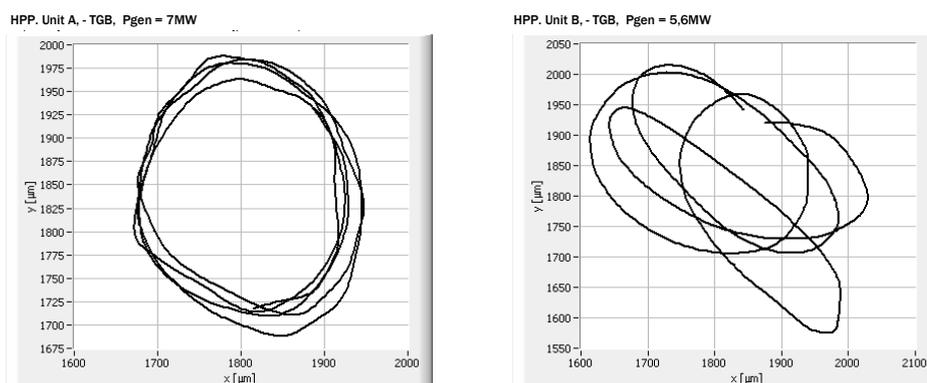
Fig. 1: Shaft runout at turbine guide bearing measured at 7 MW for unit A and at 5,6 MW for unit B
