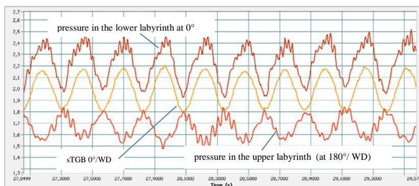
Fig. 11: Pressure measurement in the runner labyrinths
