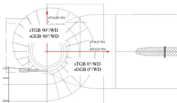
Fig. 6: Coordinate system of the shaft runout
