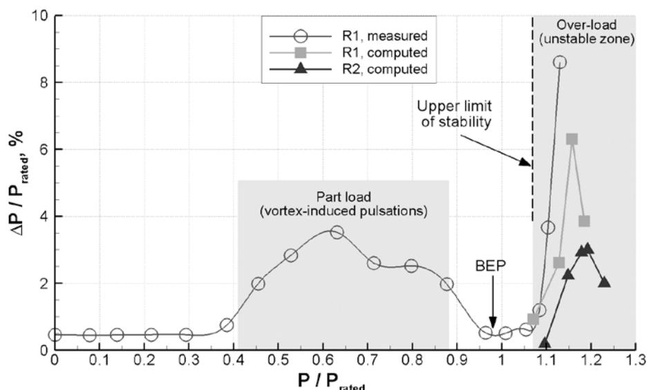
Fig. 13. Peak-to-peak amplitude of power pulsations as function of average turbine power.
