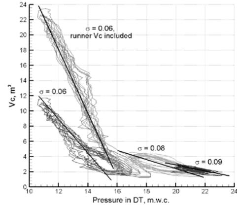
Fig. 10. Identification of cavitation compliance: cavity volume  $V_c$  against pressure in DT.
