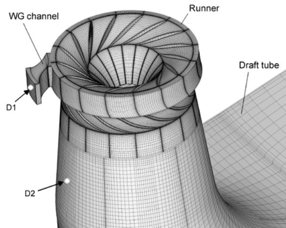
Fig.2 Mesh for "periodic WG - whole runner - draft tube" computations and monitoring points D1 (WG) and D2 (DT).
