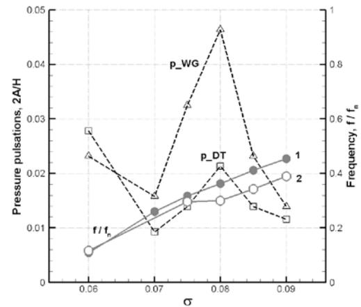
Fig. 6. Amplitude and frequency of pressure pulsations versus  $\sigma$ .
