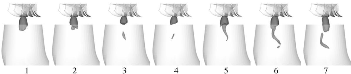
Fig. 8. Evolution of vapor cavity in runner and draft tube,  $\sigma = 0.08$ .
