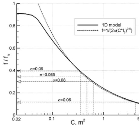
Fig. 9. First unstable frequency as function of cavitation compliance.
