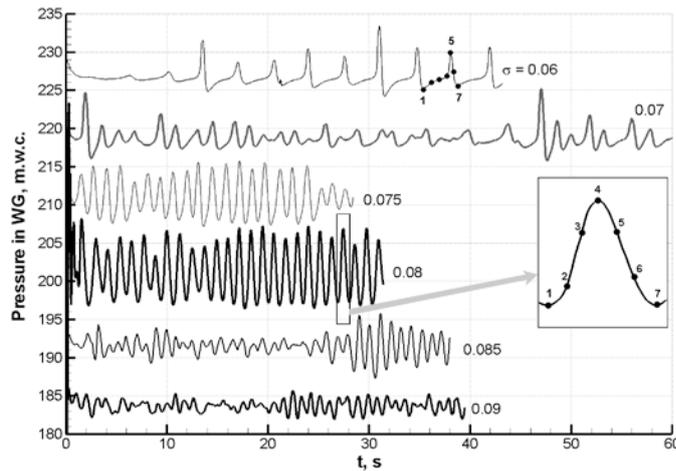
Fig. 5. Pressure pulsations in WG for various  $\sigma$ . Note, pressure levels are shifted for the sake of visualization.
