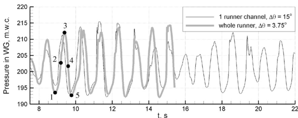
Fig. 3. Comparison of periodic and full runner computations for R1: pressure in WG.
