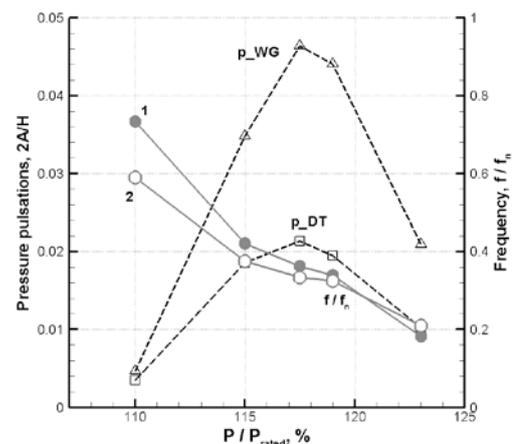
Fig. 12. Amplitude and frequency of pressure pulsations versus output power.
