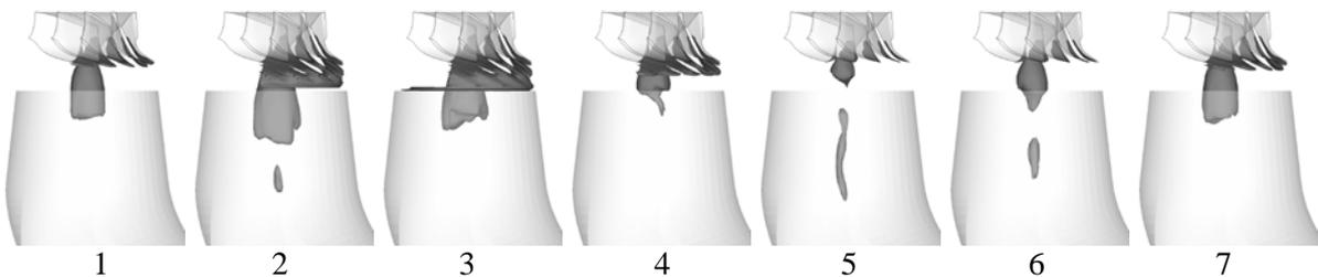
Fig. 7. Evolution of vapor cavity in runner and draft tube,  $\sigma = 0.06$ .
