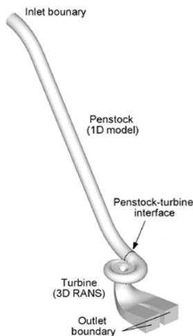
Fig.1 The concept of 1D-3D model.
