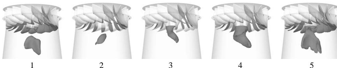
Fig. 4. Vapor cavity in runner and draft tube for 5 moments of 1 period, see Fig.3.
