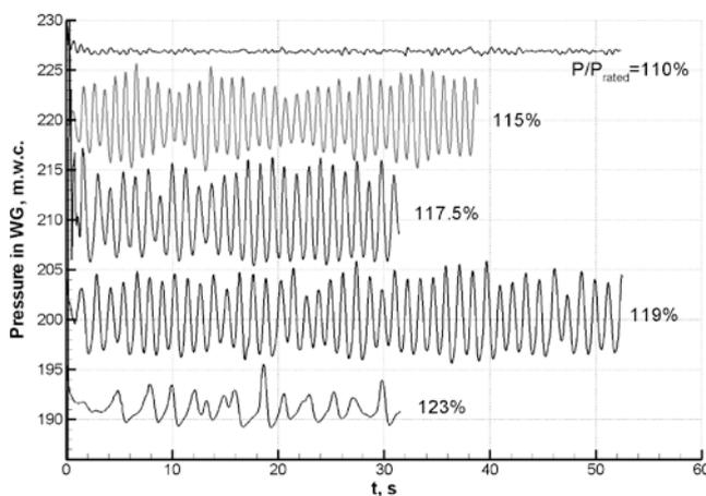
Fig. 11. Pressure pulsations in WG for various output power.
