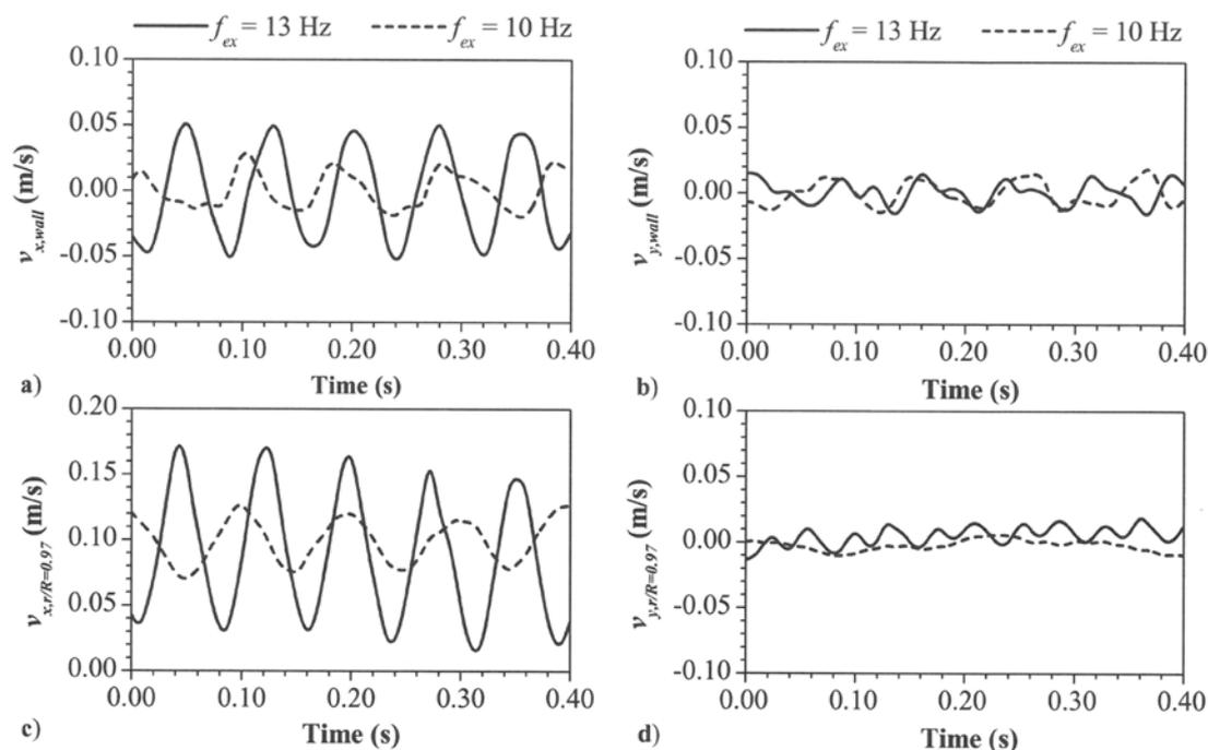
Fig. 6 Comparison of measured axial and radial velocities ( $v$ ) of the pipe wall in the PIV box and of the flow velocities at  $r/R = 0.97$  for excitation frequencies  $f_{ex} = 10$  and 13 Hz
