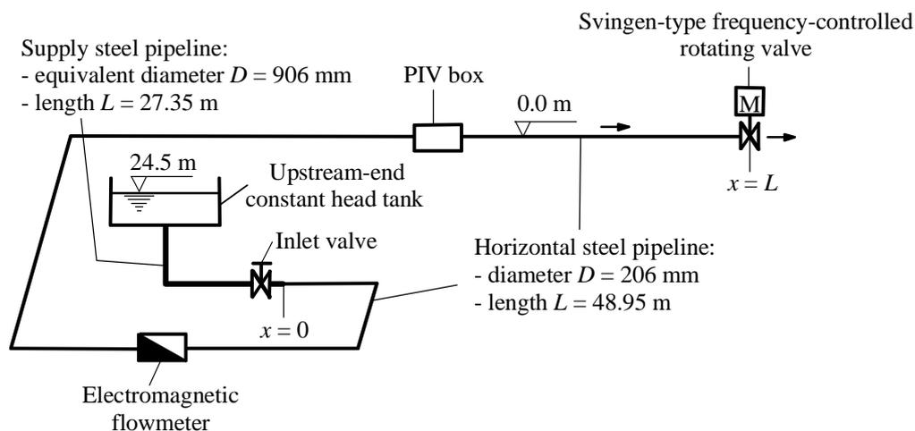
Fig.1 Test rig for oscillatory (pulsating) flow
