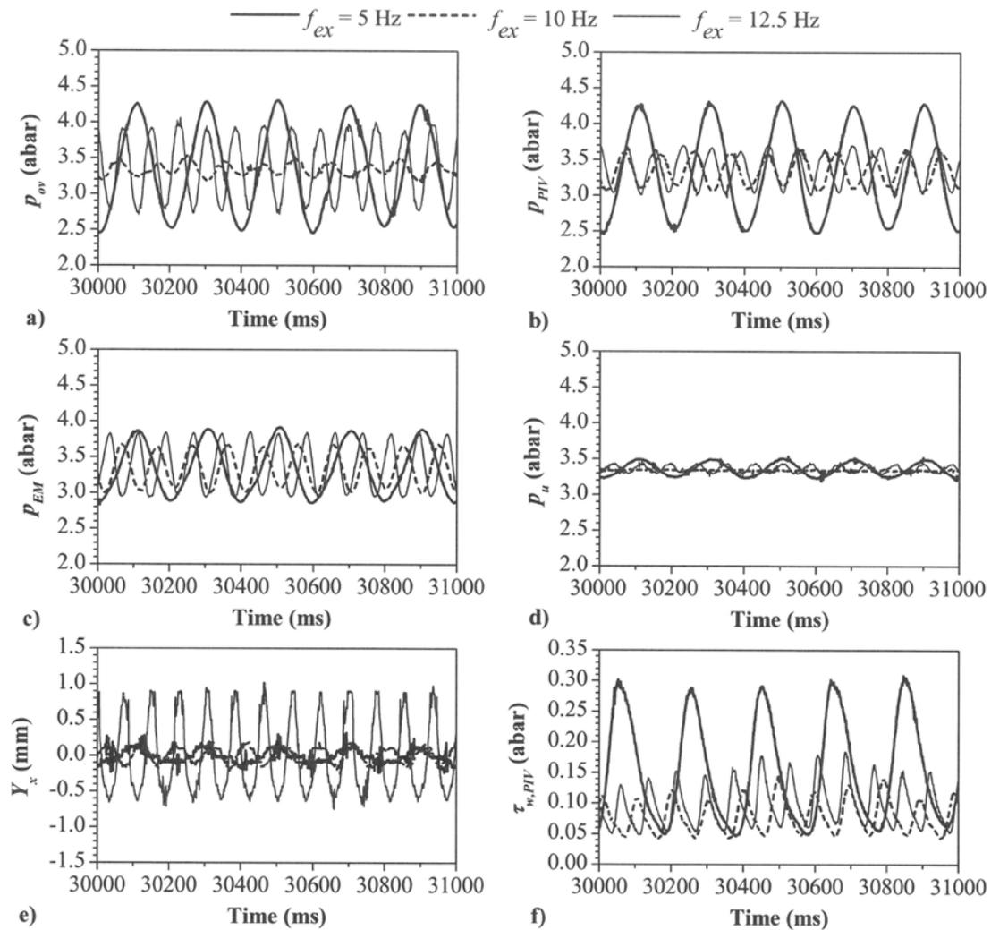
Fig. 4 Comparison of measured pressures along the horizontal test section ( $p$ , absolute), axial displacement at PIV box ( $Y_x$ ) and wall shear stresses within the PIV box ( $\tau_{w,PIV}$ ) for excitation frequencies  $f_{ex} = 5, 10$  and  $12.5$  Hz
