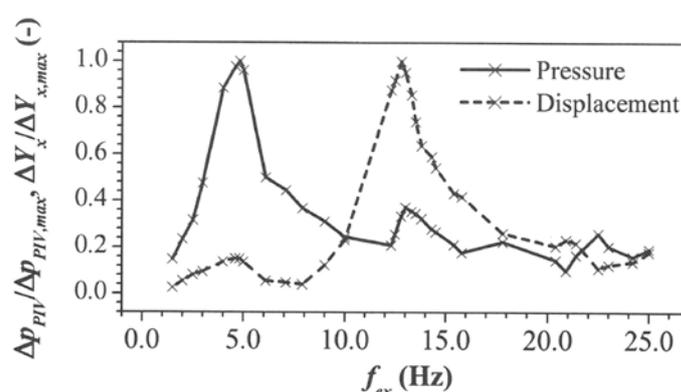
Fig. 3 Measured pressure and displacement amplitudes (normalised) at the PIV box versus frequency of oscillation of the rotating valve ( $\Delta p_{PIV,max} = 0.9$  bar;  $\Delta Y_{x,max} = 0.7$  mm)
