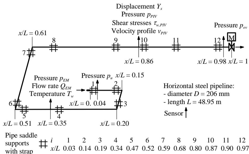
Fig.2 Layout of dynamic instruments in test section for oscillatory (pulsating) flow
