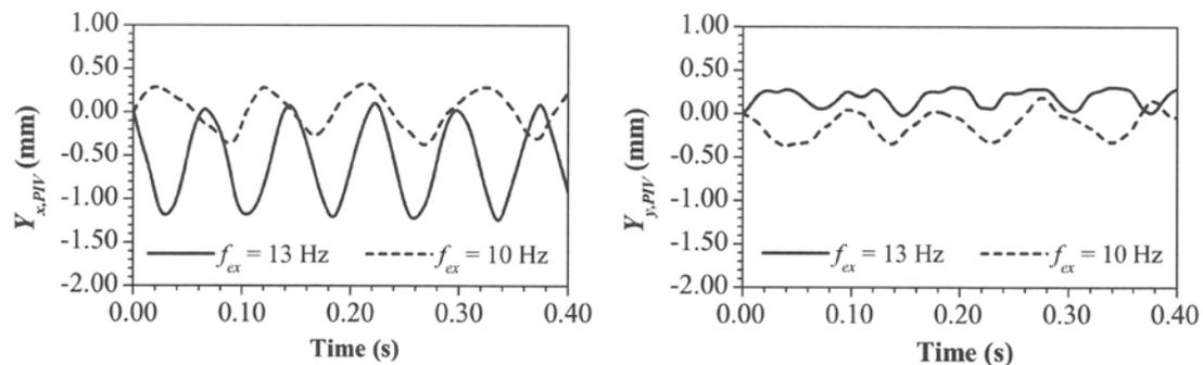
Fig. 5 Comparison of PIV images-based axial and radial displacements ( $Y$ ) within the PIV box for excitation frequencies  $f_{ex} = 10$  and  $13$  Hz
