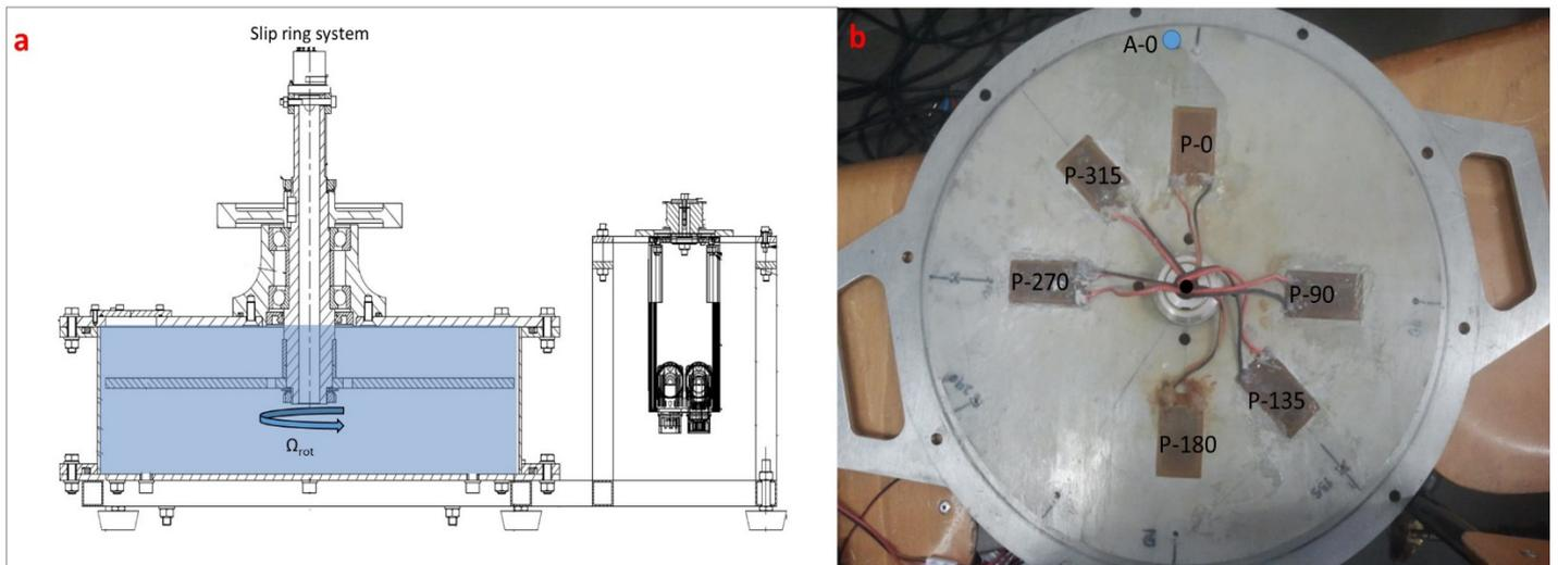
Fig.1 a) Test rig. b) Disk with attached patches and accelerometer
