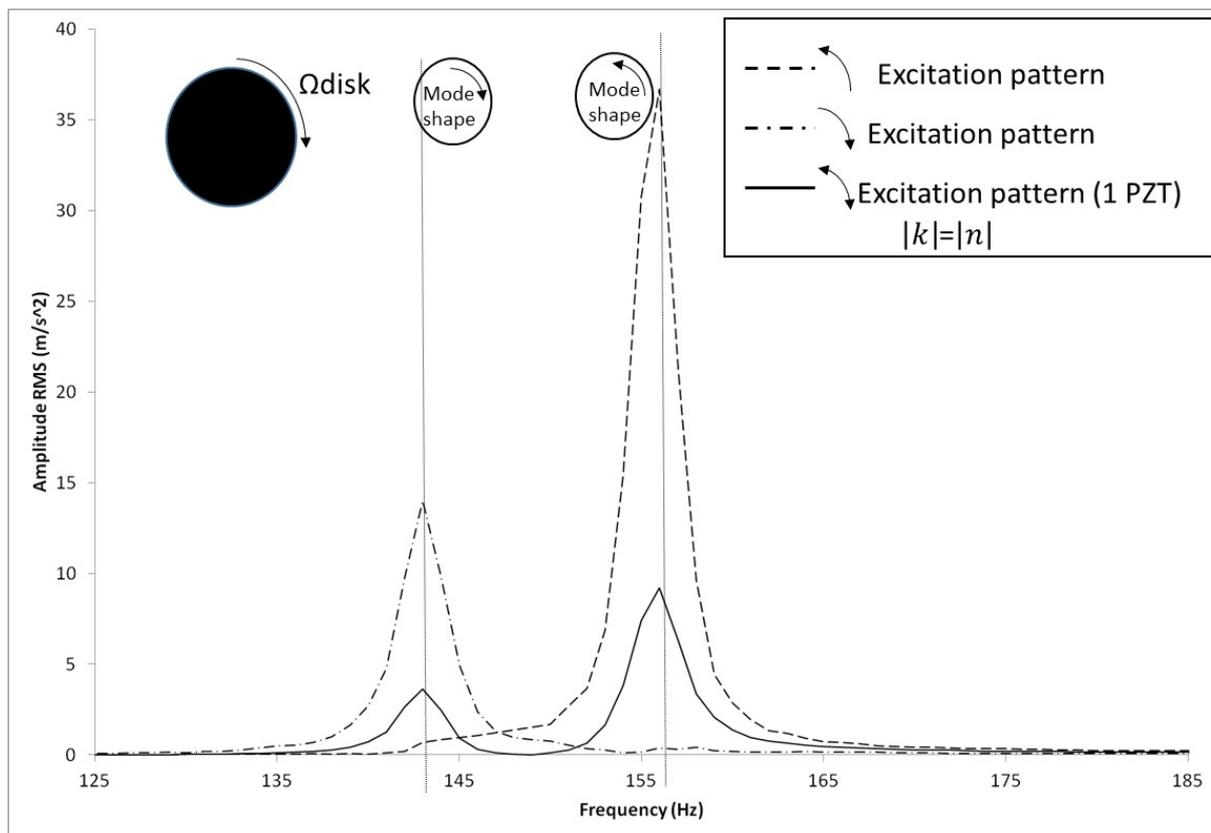
Fig.2: Excitation of the disk around the resonances  $n=\pm 2$
