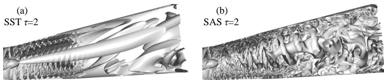
Fig.4 Isosurface of the velocity invariant  $Q=1$  for the SST and the SAS model
