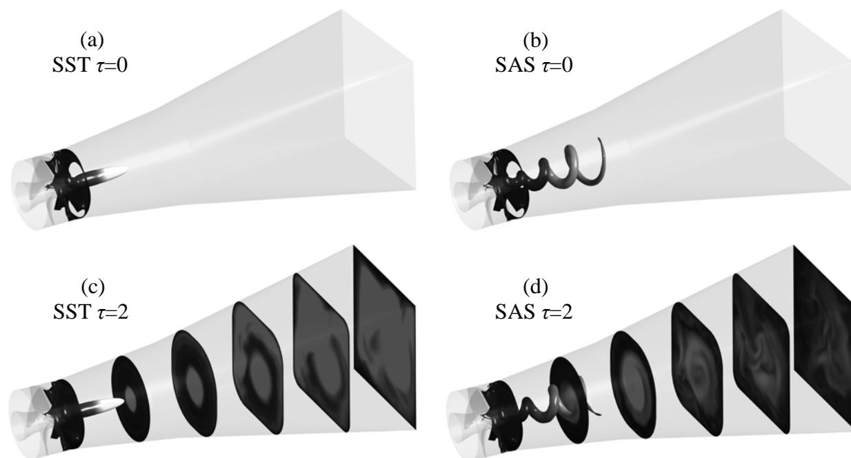
*Fig.3 Shape of the vortex rope in the draft tube for the SST and the SAS model with and without runner gap with additional planes in the draft tube (c), (d) colored by the viscosity ratio 0-2000*
