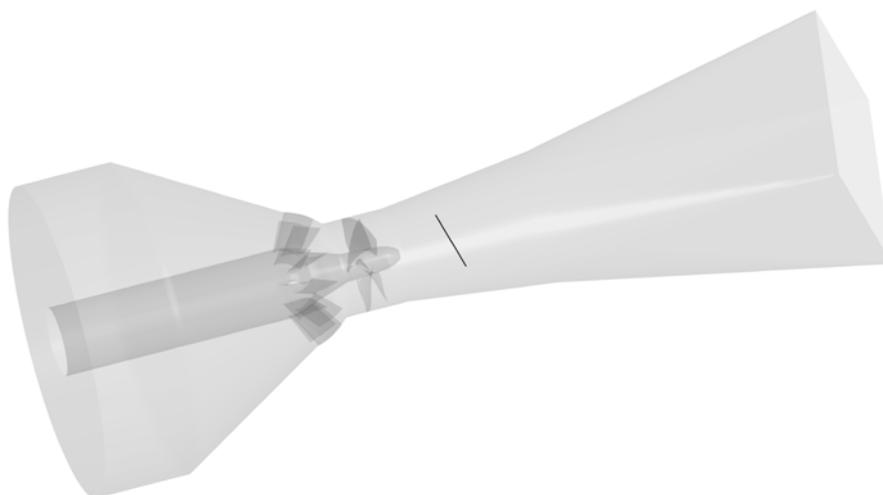
Fig.1 Hydraulic contour of the propeller turbine with marked evaluation line for the velocity profile
