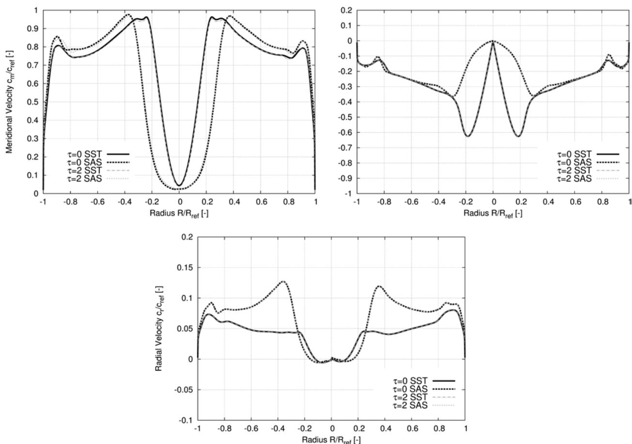
Fig.2 Time averaged velocity profiles for the SST and the SAS model with and without runner gap
