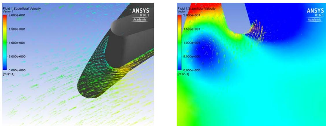
Fig. 8 CFD calculation of inlet recirculation
