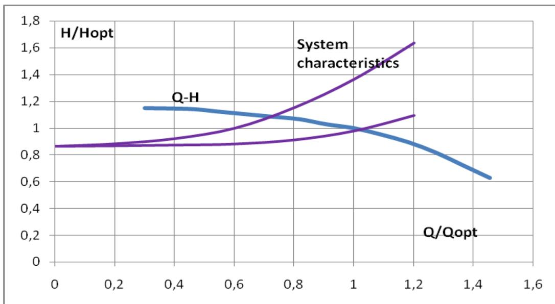
Fig.2 Dimensionless characteristic curve of existing pump and system characteristic
