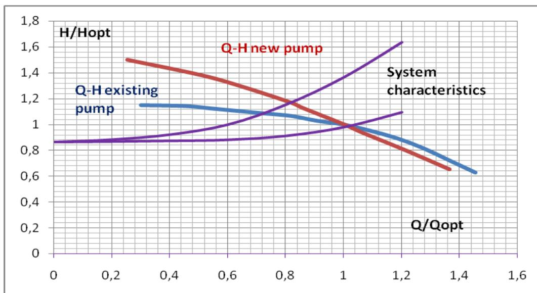
Fig.5 Dimensionless Q-H Characteristic of the new pump compare with existing one
