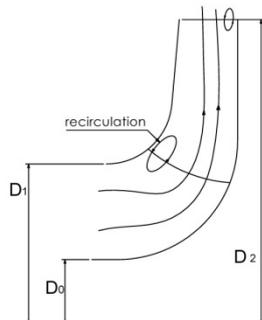
Fig. 1 Suction recirculation at the inlet
