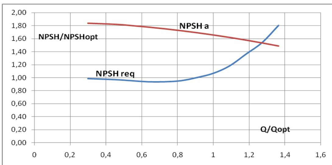
Fig.3 Dimensionless characteristic of NPSH req and NPSH a
