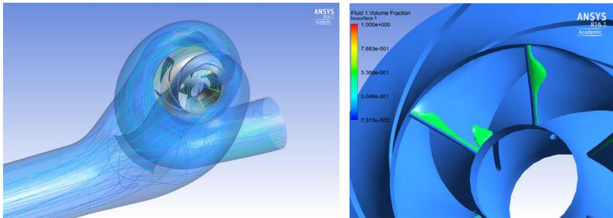
Fig. 7 CFD calculation of bubble formation
