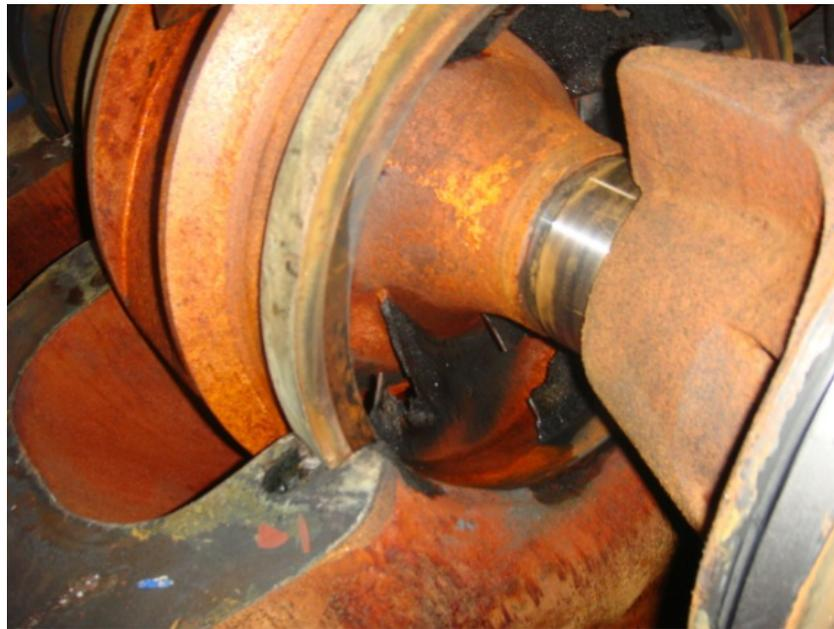
Fig.4 Cavitation damage due to the recirculation
