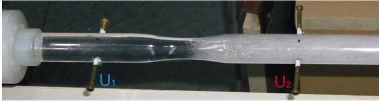
Fig. 6 The cavitation tube with point electrodes
