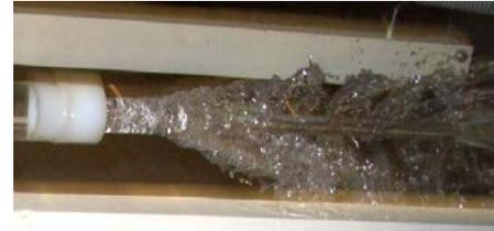
Fig. 7 Structure of the cavitation caverns
