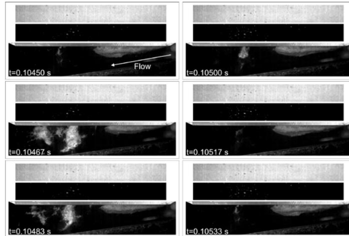
Fig. 2: Instantaneous image of the aluminum foil (top images), measured damage of the foil up to this instant (middle images) and instantaneous image of cavitation (bottom images) [9]. The flow is from the right to the left.
