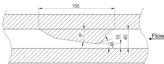
Fig. 1: The Venturi geometry.
