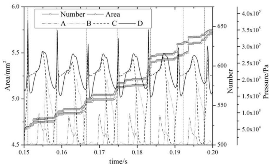
Fig. 4: Number of pits, integral damage extent and absolute pressure at the monitor points A, B, C, and D as a function of time. At cavitation number  $\sigma=1.48$  and velocity at the Venturi throat  $v=24.7$  m/s, Reynolds number  $Re=247000$ .
