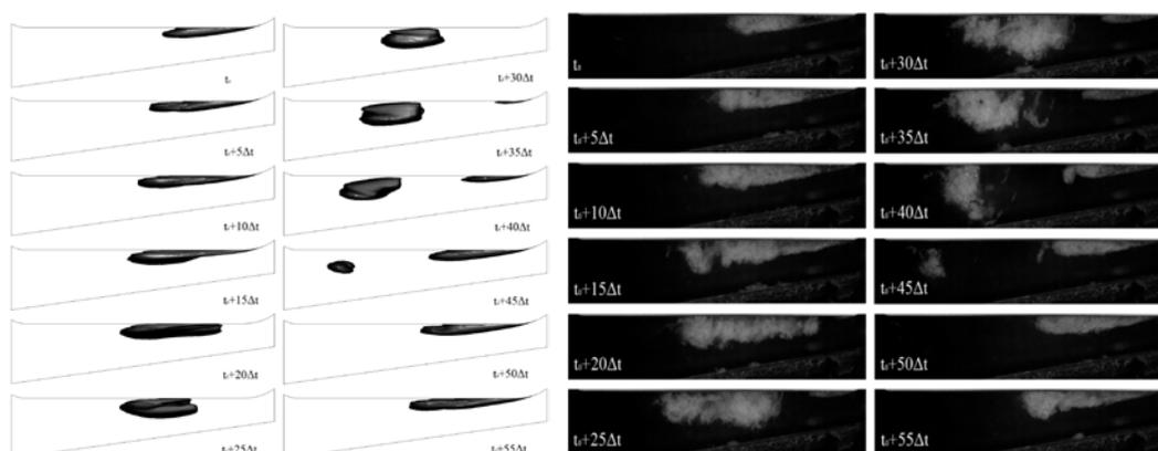
Fig. 3: Simulated (left) and observed (right) cavitation structure evolution, the flow direction is from right to left.  $\sigma=1.48$  and  $v=24.7$  m/s.
