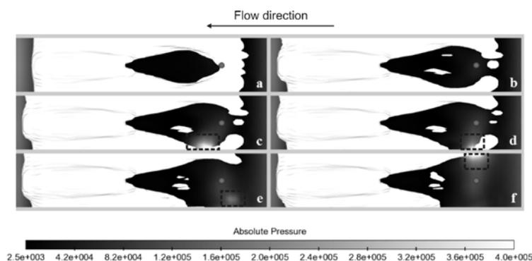
Fig. 6: Absolute pressure on Venturi surface at times a to f during cavitation shedding process.  $\sigma=1.48$  and  $v=24.7\text{m/s}$ . The flow direction is from right to left.
