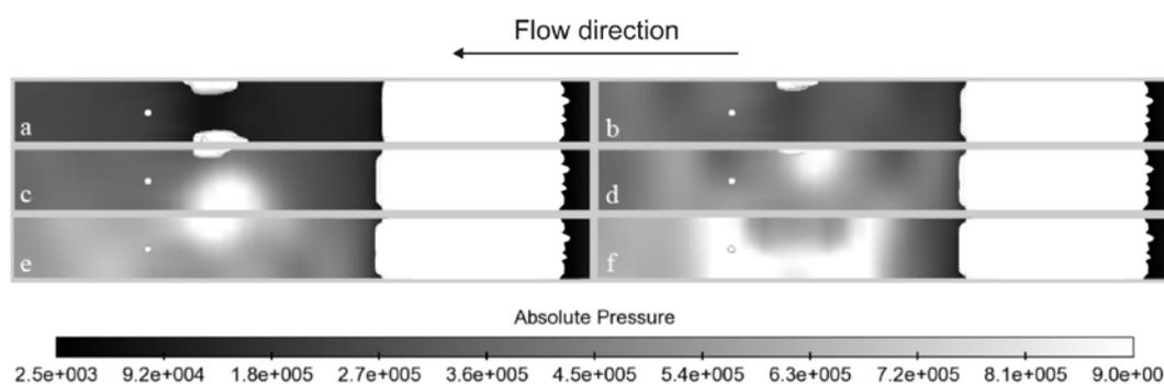
Fig. 5: Absolute pressure at the Venturi surface at times a to f during cavitation cloud collapse.  $\sigma=1.48$  and  $v=24.7$  m/s. The flow direction is from right to left.
