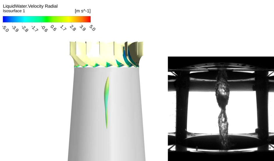
Fig 4. Left: Iso-surface of the gas volume fraction ( $r_g = 0.1$ ).
