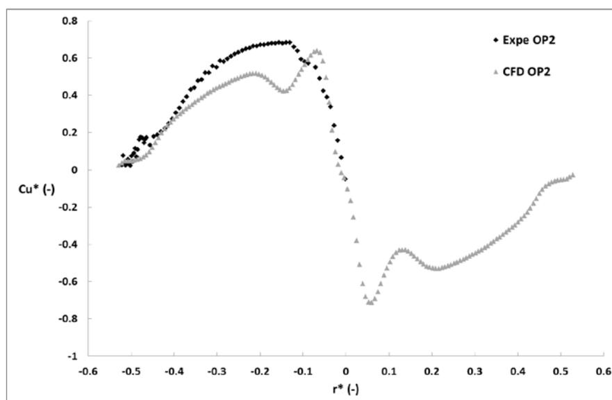
Fig 5: Dimensionless circumferential velocity  $Cu^*$  in the upper section.
