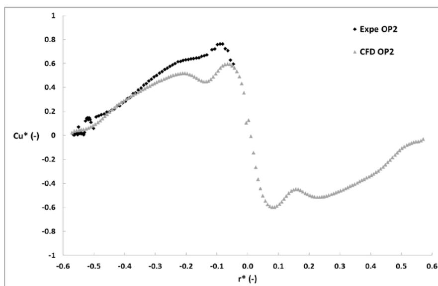
Fig 6: Dimensionless circumferential velocity  $Cu^*$  in the lower section.
