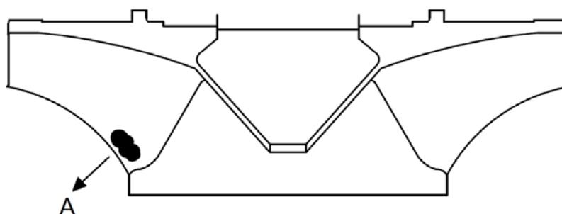
Figure 2. Schematics of occurrence of cavitation in pump mode (area A)
