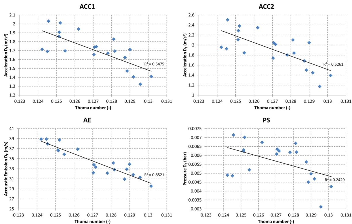
Figure 5. Discharge coefficient cavitation estimator ( $D_E$ ) for different cavitation sensors
