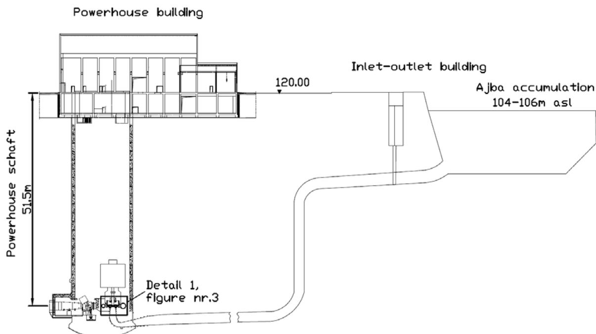
Figure 1. The power house of pump- storage hydro power plant Avče
