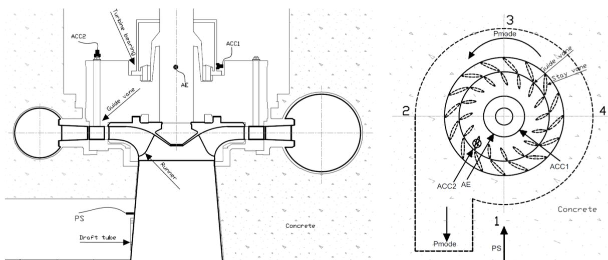
Figure 3. Installation of sensors (detail 1 of the fig 1) showing: (left) view from side; (right) view from top (AE - acoustic emission sensor, ACC1 and ACC2 accelerometers 1 and 2, PS - pressure sensor).
