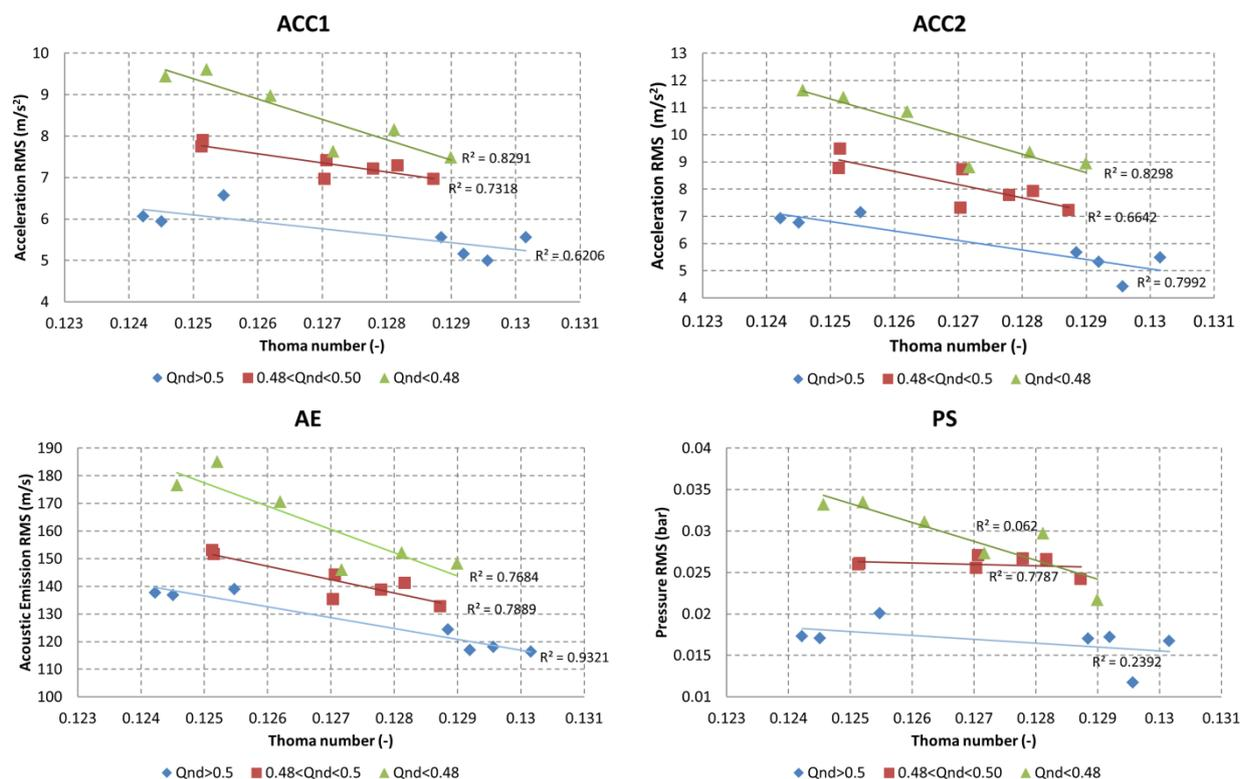
Figure 4. Results of measurements of vibrations, acoustic emission and pressure fluctuations, showing dependence of measured variables on three intervals of discharge coefficients.
