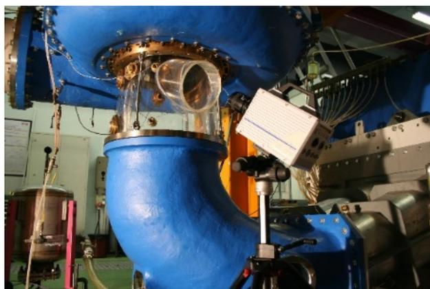
*Fig. 1 Experimental setup for high speed visualization of inter-blade cavitation vortices*
