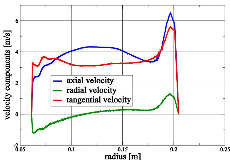
Fig.2 Velocity components distribution on inlet section of the draft tube.
