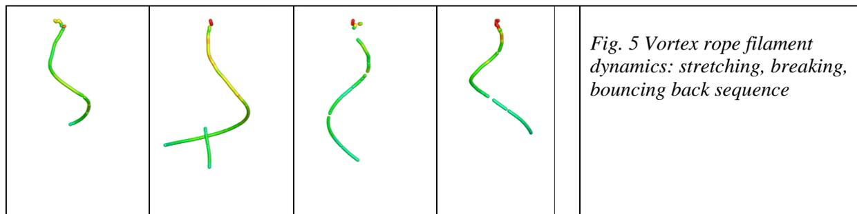
Figure 5 shows significant changes in the vortex rope shape as it rotates with the precession frequency. One can identify an elongation phase, where the pitch increases and the vortex filament is stretched. Then, at the end of this stretching phase the vortex filament breaks up and the segment attached to the runner crown bounces back reaching a small pitch. The cycle is repeated with a smaller frequency than the precession frequency.
