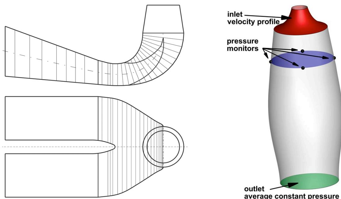
Fig. 1 The elbow draft tube (left) and the hydraulically equivalent axisymmetric domain (right).
