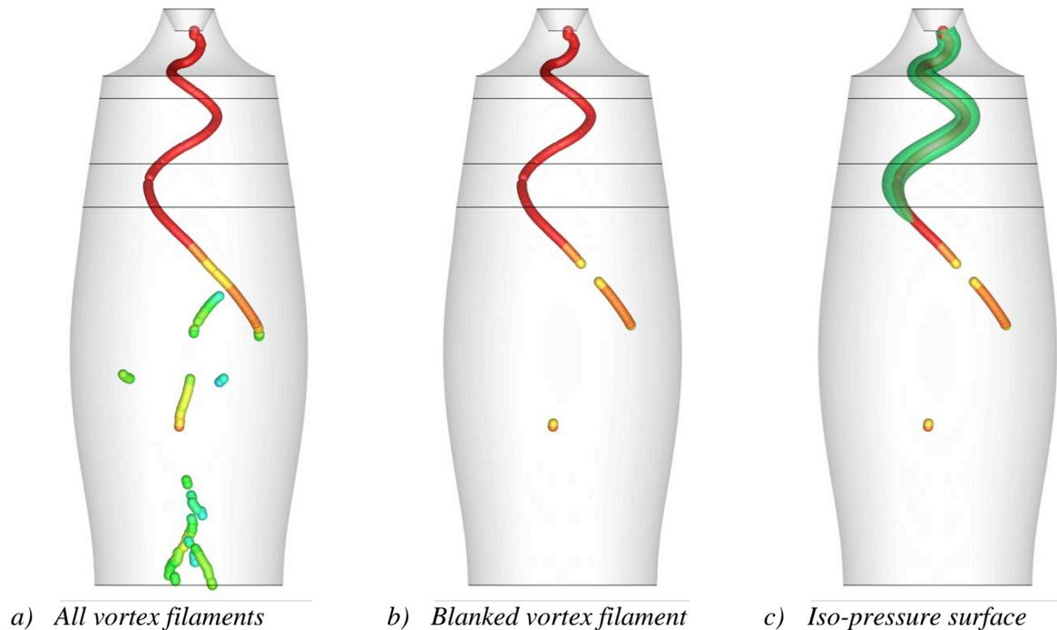
Fig. 3 Vortex filament extraction and correlation with iso-pressure surface.
