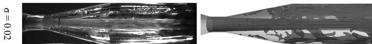
Fig. 11 Supercavitation regime, experiment (left,) numerical simulation with contour corresponding to 99 % of liquid water (right)
