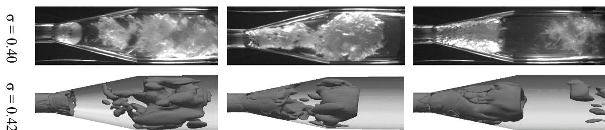
Fig. 10 Comparison of the numerical results with high speed video records.
