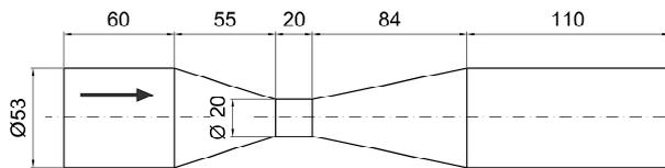
Fig. 1: Dimensions of the converging-diverging nozzle
