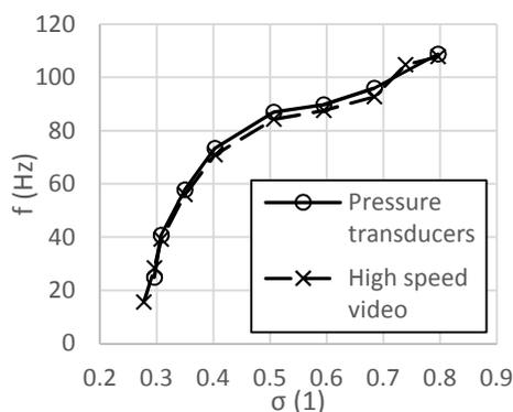
Fig. 5 Analysis of the pressure fluctuations: open vessel
