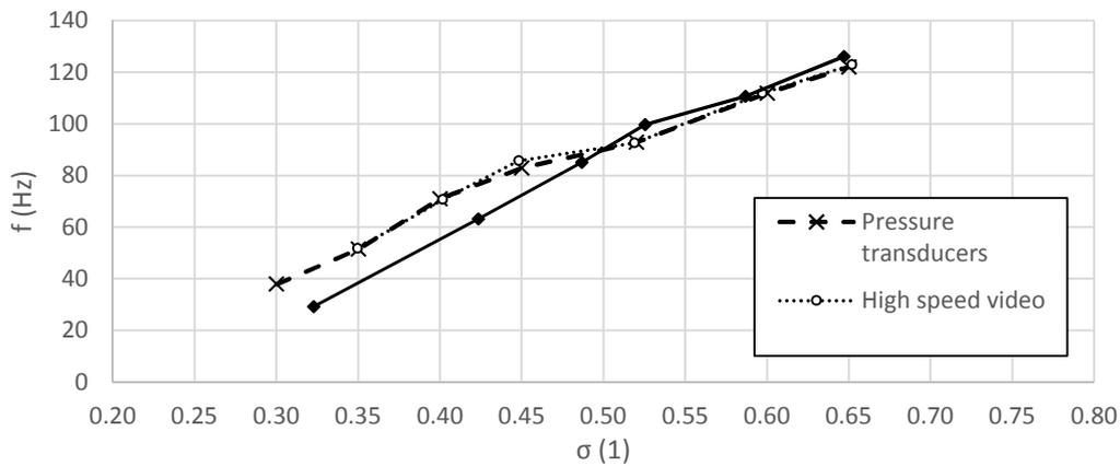
Fig. 9 Comparison of dominant frequencies for flow rate 7l/s
